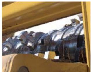
Hardface weld surfacing to extend the life of the rotor
