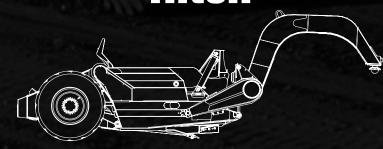
Weight distribution is 25/75% tractor/scraper to maximize tractor longevity. The tractor tow model is best for light soils or high moisture content soils.
